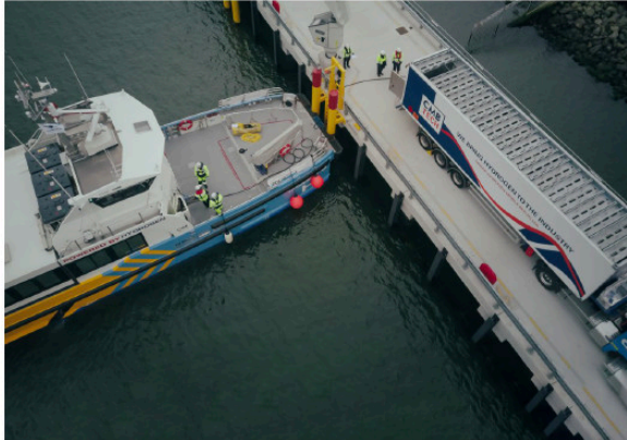
CMB.TECH H2 tube trailer bunkering Hydrocat (H 2 dual fuel crew transfer vessel)
