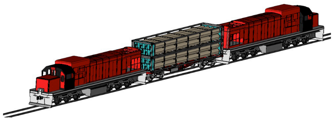
Figure 3: Locomotive consist concept for the H2 DF Locomotive project
